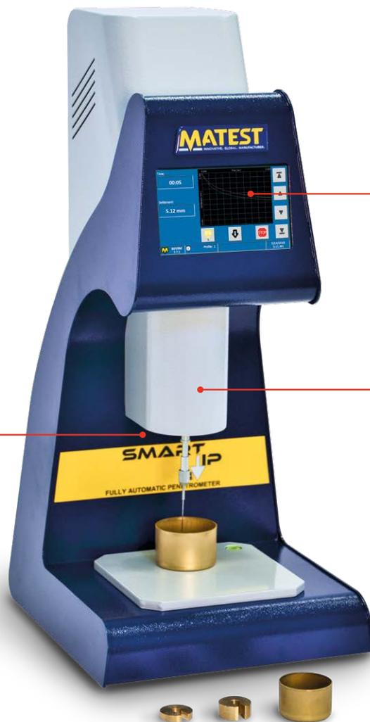
The instrument automatically reaches the contact point before starting the test and the penetration result is measured by a high performance contactless displacement transducer.
