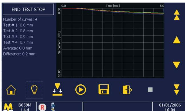
Real time penetration/time graph, test temperature and average result from a batch of tests.
